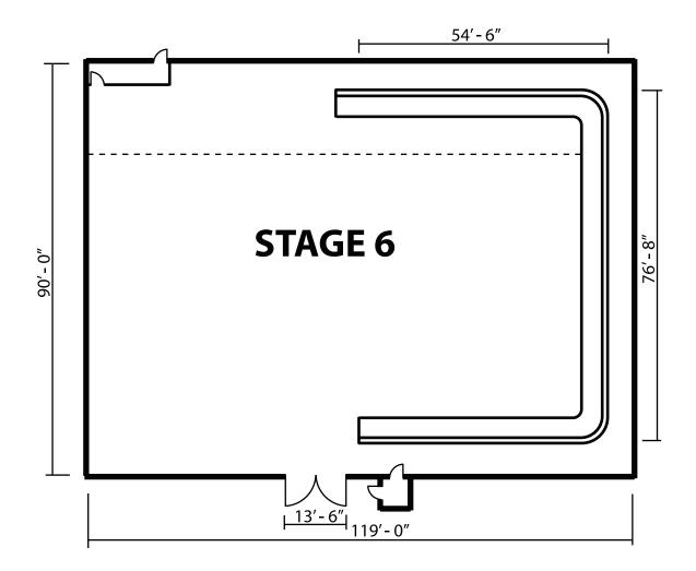
LENGTH: II9' WIDTH: 90' HEIGHT: Main = 26'6"; low = 20' AREA SQUARE-FEET: 10,710 FOR SYNC SOUND: Yes AUDIENCE-RATED: No CAT WALKS: Yes FLOORS: Wood over slab small pit DRIVE-IN: Yes AIR CONDITIONING: Red-lighted units AC POWER: 3600 amps DC POWER: 3600 amps DOOR SIZE: Ht. 18' Wd. 13'6" HARD-COVED CYC: Three-wall VIDEO CONTROL ROOM CONNECTIVITY: No
