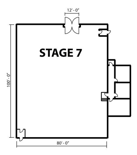
LENGTH: 80' WIDTH: 100' HEIGHT: 24' AREA SQUARE-FEET: 8,000 FOR SYNC SOUND: Yes AUDIENCE-RATED: 250 + crew of 49 CAT WALKS: Yes FLOORS: Wood over slab DRIVE-IN: Yes AIR CONDITIONING: 80 tons/silent AC POWER: 2400 amps DC POWER: 1000 amps DOOR SIZE: Ht. 16'11"Wd. 11' HARD-COVED CYC: No VIDEO CONTROL ROOM CONNECTIVITY: Yes; triax & audio break-outs/tech power
